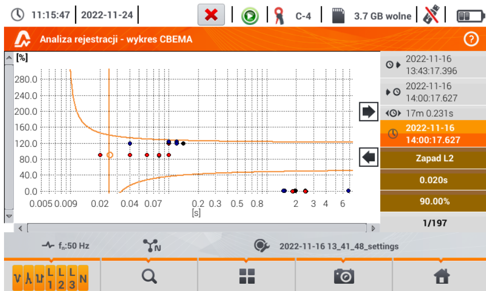
Fig. 5.27. Recording analysis – CBEMA graph
