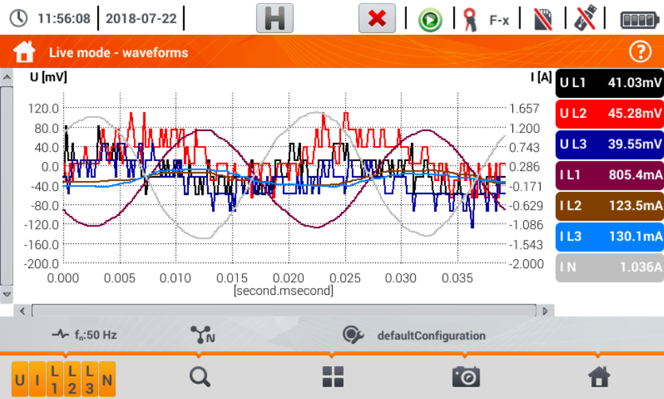
Fig. 5.13. "Live" mode - waveforms
